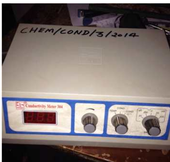
CONDUCTIVITY METER Rs. 12075x3= 36225 To determine the value of conductivity of any solvent
