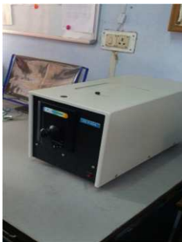
SPECTROPHOTOMETER Rs. 332,719 For measuring colour intensity, hue, value and other parameters of dyed fabrics or liquids
