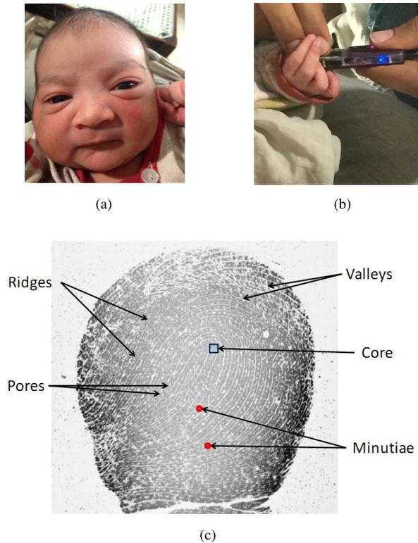
Fig. 1. Fingerprint capture of a 6 hours old child using the custom 1,270 ppi fingerprint reader designed by NEC [3]. (a) Face image of the child, (b) the fingerprint capture process, and (c) the captured left thumb print image with annotated features (ridges and valleys, core, minutiae, and pores).
