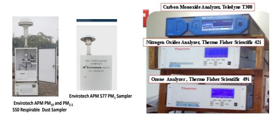
Figure 31: PM Samplers and Trace Gas On-Line Analysers at DEI
