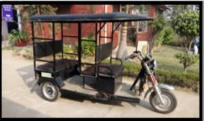
Figure 33: Electric Golf Cart and e-rickshaw developed by B. Voc. Automobile Students
