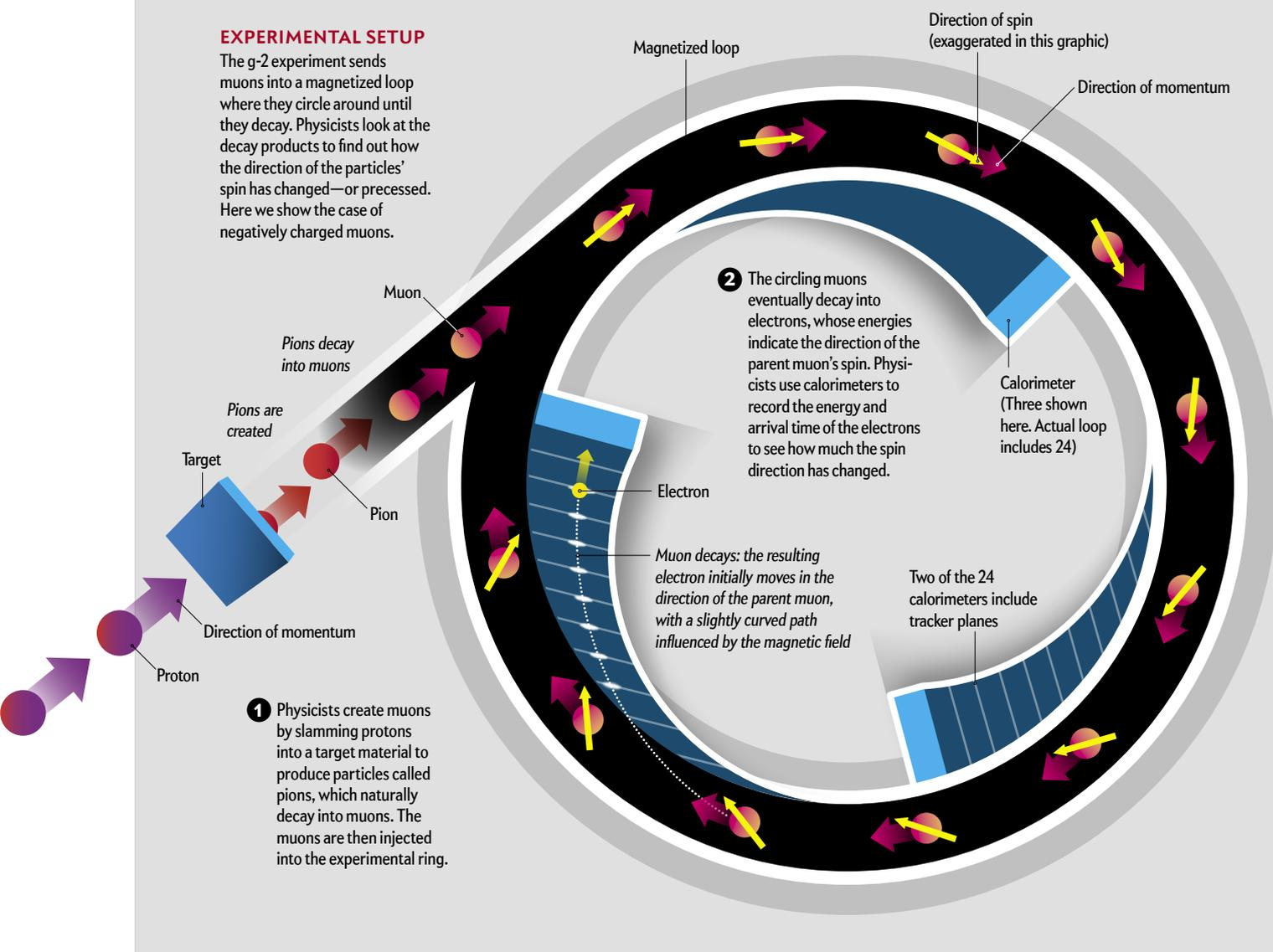
**1** Physicists create muons by slamming protons into a target material to produce particles called pions, which naturally decay into muons. The muons are then injected into the experimental ring.
