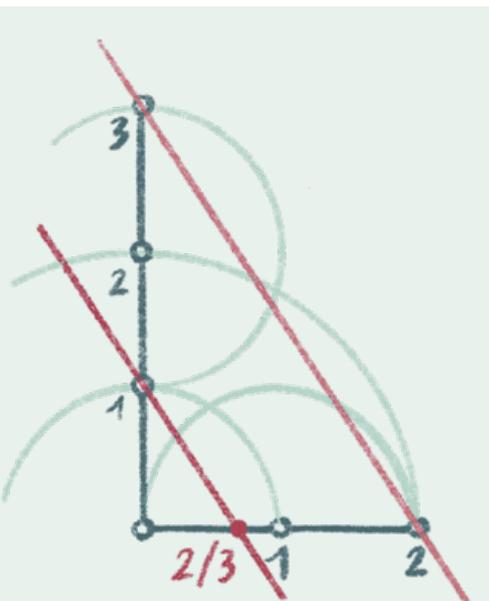
**Step 4:** Use a straightedge to draw a line through point 2 on the horizontal axis and point 3 on the vertical axis. Use compass to make two perpendicular lines to construct a parallel line between the vertical point 1 and the position of 2/3 on the horizontal axis.
