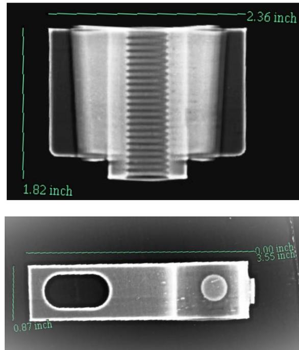
**Figure 4:** CT X-ray scans of parts #2 and #1 produced for a company
