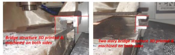
**Figure 7:** Hybrid technology allows 3D print and machining single or multi-store bridges
