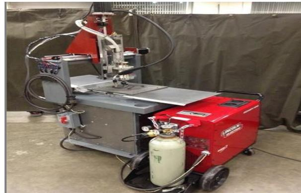
**Figure 3:** Hybrid 3D Metal printing prototype
