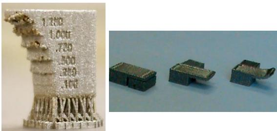
**Figure 4:** Existing metal 3D printing problems-overhang structures [11].
