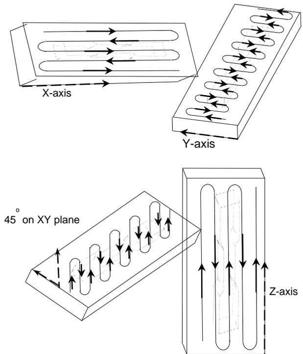
**Figure 1:** Deposition directions: along on X –axis, across on Y-axis, on 45°, and on vertical Z-axis
