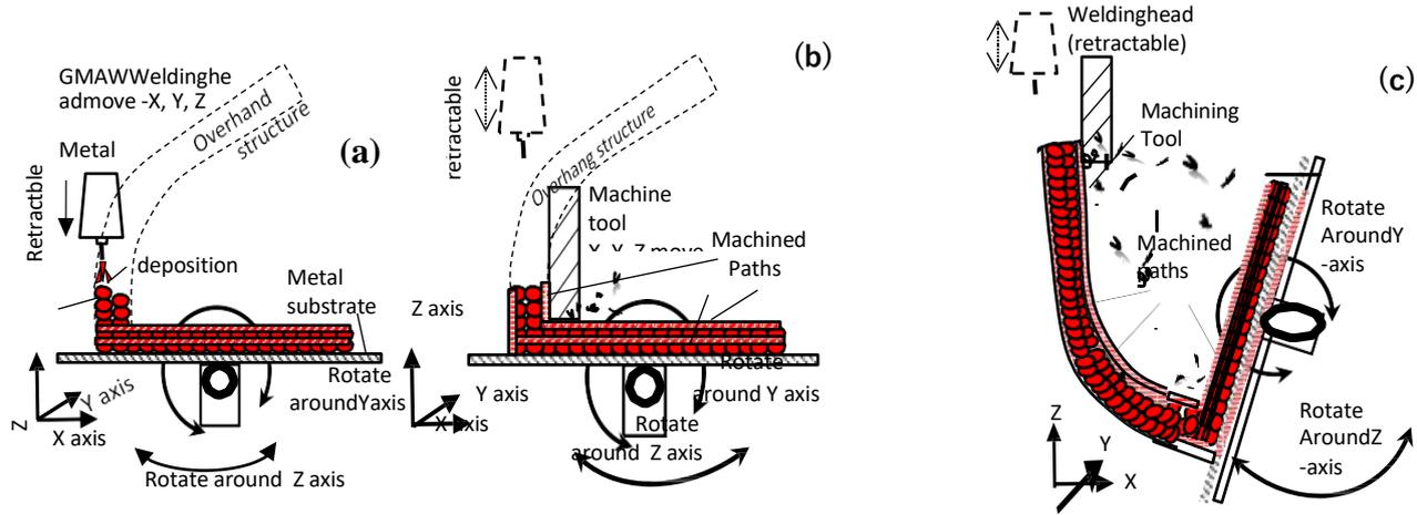
**Figure 2 (a, b, c):** 5 axis hybrid 3D printing-MIG welding deposition and CNC machining of overhang structure
