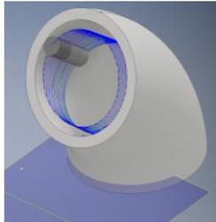
**Figure 9:** Hybrid 3D design of toroidal surface machined inside/outside
