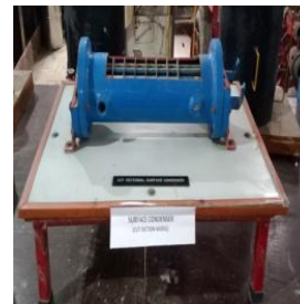
Model of Surface Condenser
