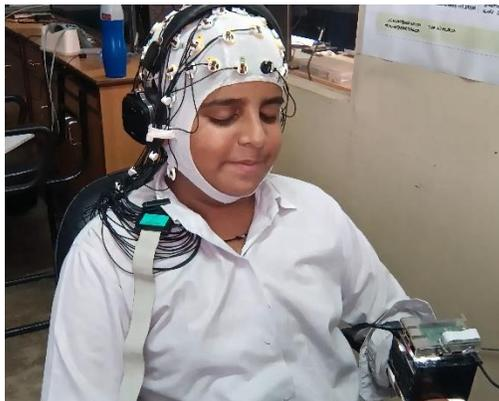
Fig. 4. Subject wearing goosebumps measuring device with 64 channel wet EEG cap.
