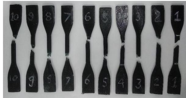
**Fig. 11. Specimen after tensile test**
