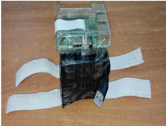
Fig.1. Representative picture of the goosebump measuring device fabricated in our lab. Parts of the device: raspberry pi settle on a black-colored stencil fitted with a camera on the inside (not shown in the picture) with white-colored straps to wear the device on hand.
