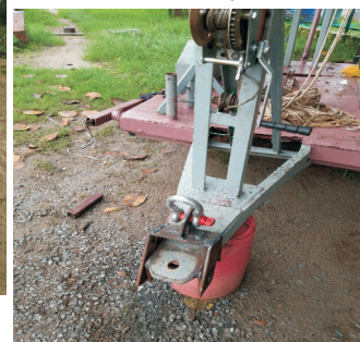
Fig. 7. Towing Bracket fabricated on the trailer
