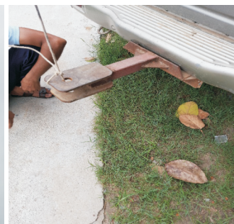
Fig. 6. Fabricated Towing Hitch on Scorpio
