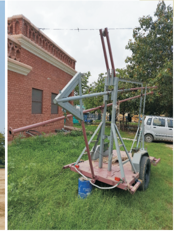
Fig. 4. Trailer with mast system installed
