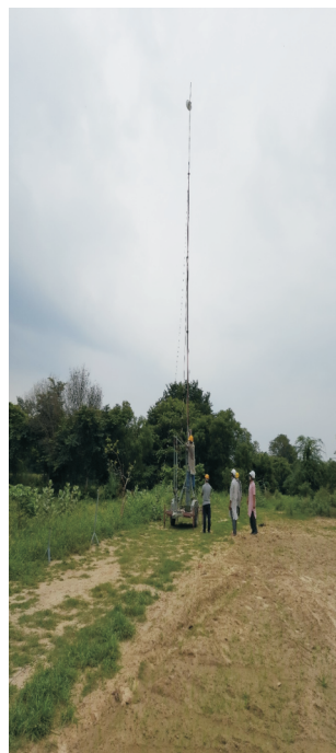
Fig. 5. Trailer mast with extended telescopic length 55ft at Sikandarpur Pulia No.2
