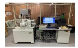
• **Thermal Desorption Unit (TDU)** worth Rs. 35 lakes procured under the FIST grant is under installation hyphenated to GC-MS. This combined unit would enable simultaneous sampling and analysis of volatile organic compounds present in the gas phase.
